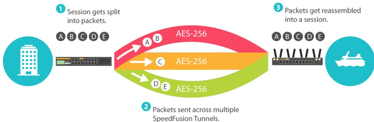
**SpeedFusion creates an additional layer of security by routing sub-packets of traffic across multiple physical media types across different telecommunication providers.**
